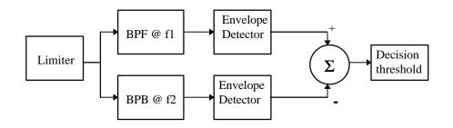
This model suggests that non-coherent FSK modulation can be treated as two ASK signals, one at frequency f1 and the other at frequency f2. Since the limiter theoretically keeps the amplitude of the signals at f1 and f2 constant, the probability distribution appears as follows:
