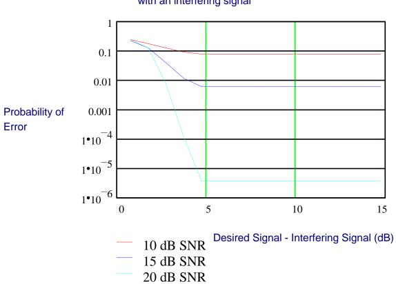
4.77 dB delta ASK signal with an interfering signal
