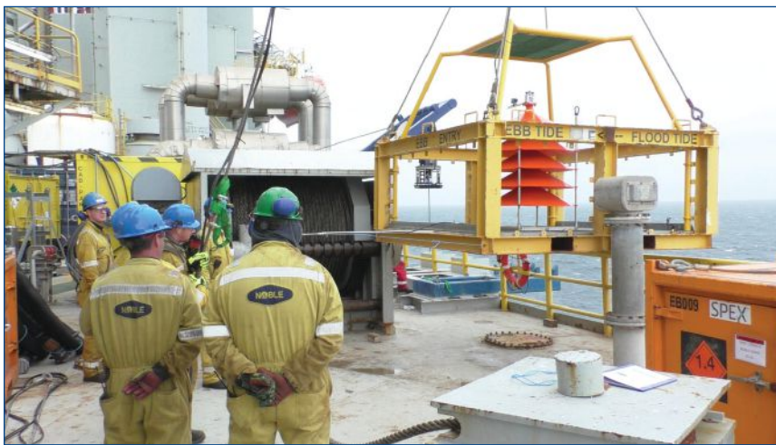
(From top to bottom) Sentinel Subsea's CTO Dr. Andrew Jaffrey with the alert beacon. The WellSentinel test rig before being lowered to the seabed off the Noble Hans Deul. The WellSentinel Coral design showing the alert beacon being released to the surface.
