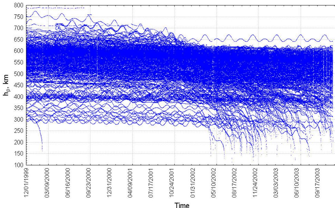
**Figure 1. Time-Altitude Distribution of Ballistic Coefficient Estimates (for all SOs)**
