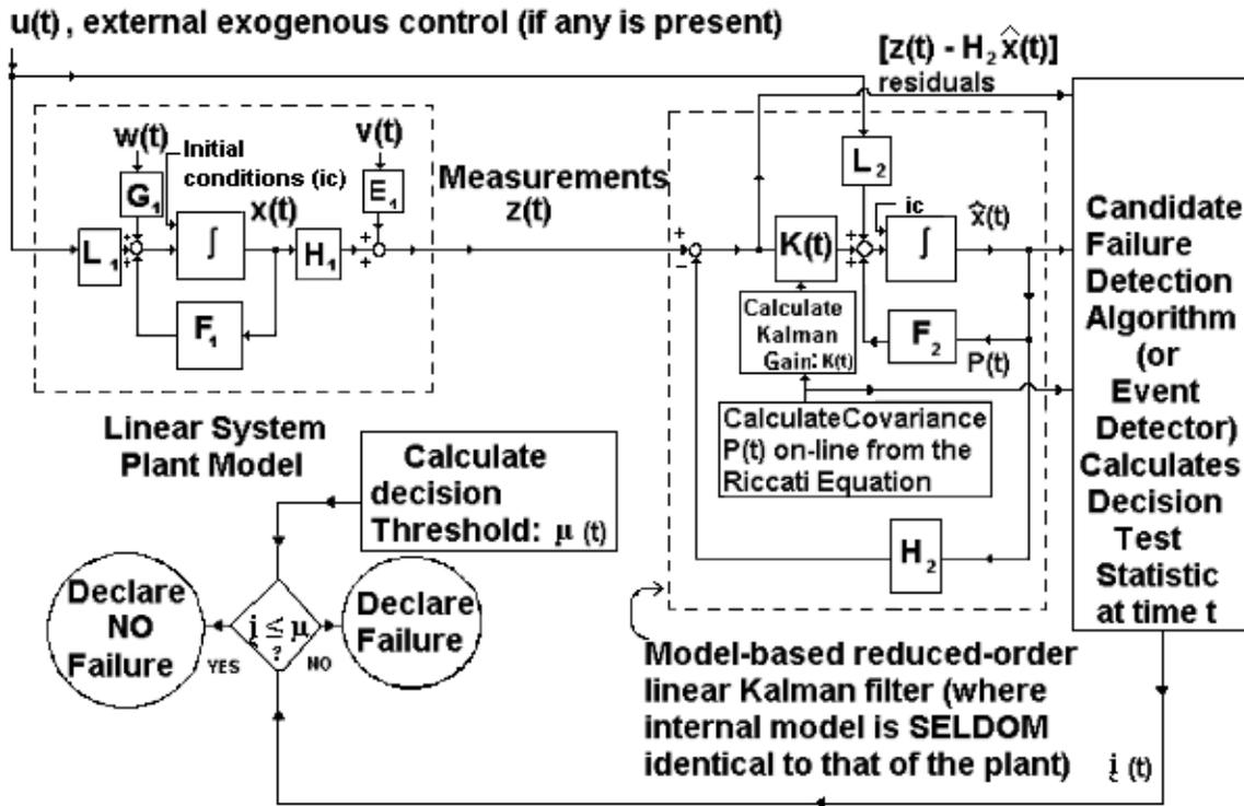
Fig. 1. Continuous-Time Summary of Navigation Failure Detection Algorithm's Structural Operations on Outputs of Linear System Plant Outfitted with a Linear Kalman Filter
