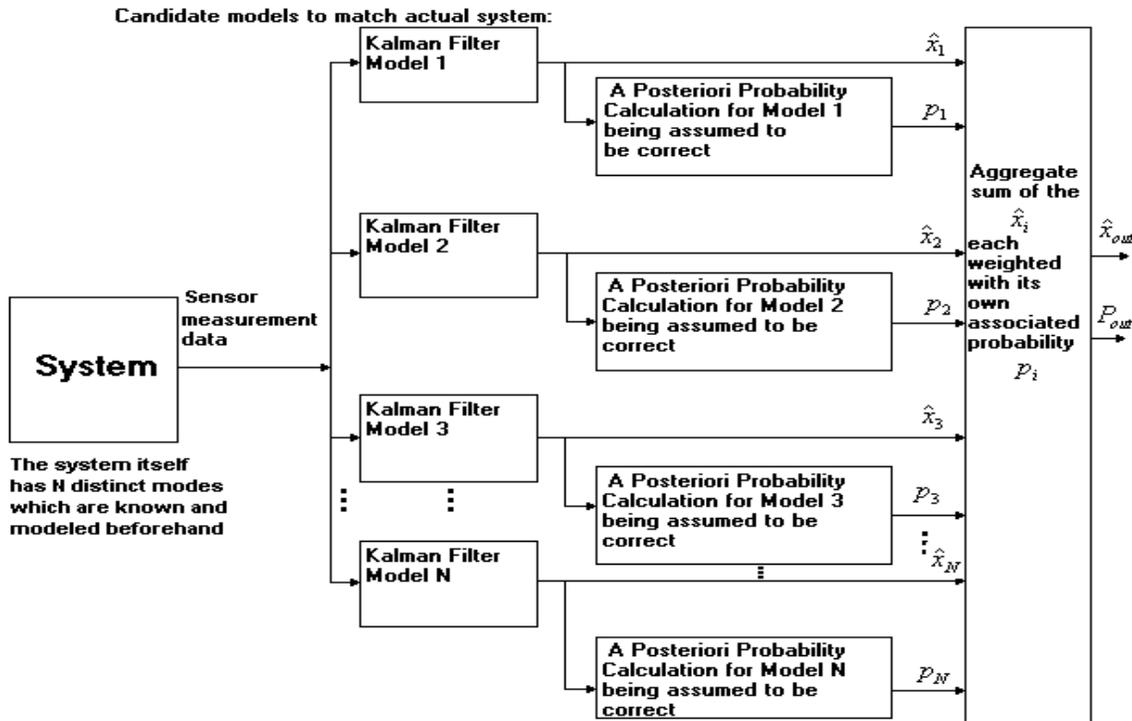
Fig. 2. Parallel bank-of-filters structure of Interactive Multiple Model (IMM) formulation for tracking systems that jump between a finite number, N, of alternative but specified modes (which have been modeled a priori)
