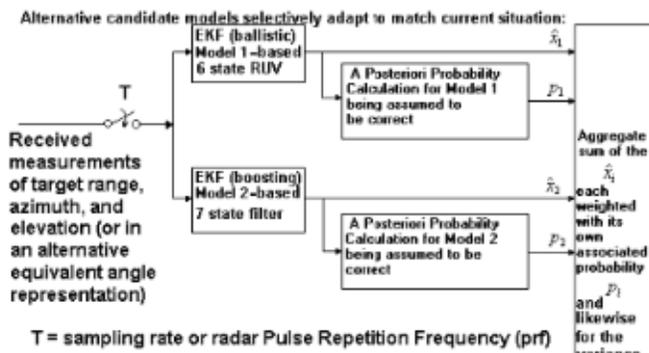
Fig. 3. A preliminary hypothesized IMM structure for tracking objects via radar as they transition between exoatmospheric and indoatmospheric regime or vice-versa (where the two filters have different state sizes)
